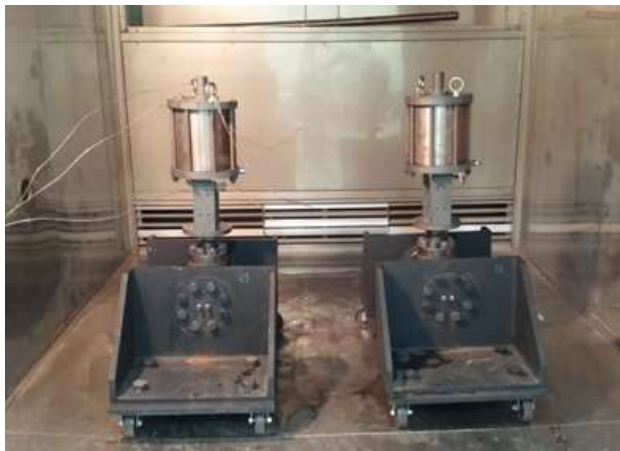
Fig. 2. Thermal aging chamber and test valve
